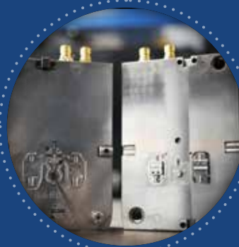
1+1+1 family tool for the lock button top, bottom, and cap
